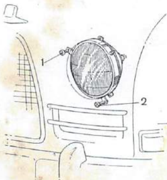
Fig. 29. Screws for adjusting Headlights 1. Horizontal adjustment 2. Vertical adjustment
